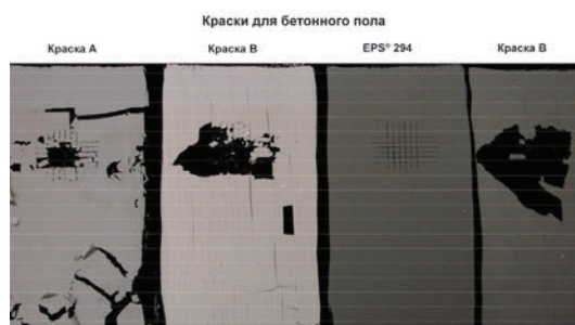
FIGURE 11. EPS® 294 COMPARED TO COMPETITIVE PAINTS AFTER 2 HOUR WATER IMMERSION AND CROSSCUT/TAPE ADHESION TEST
